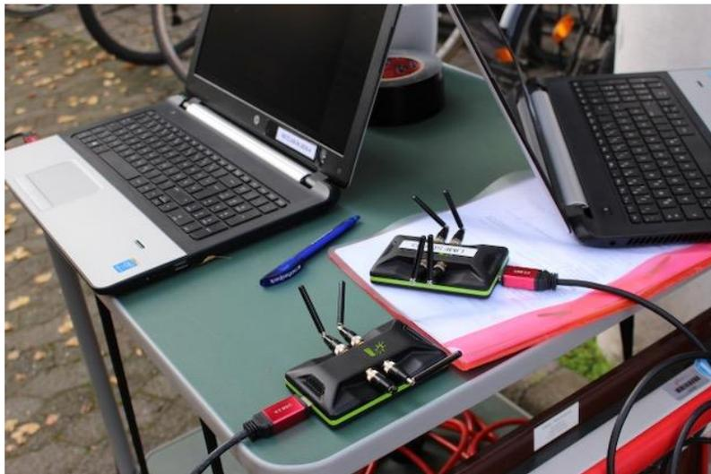
Simple setup with two LimeSDRs
