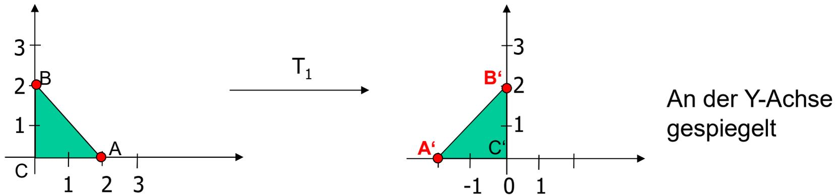
$$\vec{A}' = T_1 \cdot \vec{A} = \begin{pmatrix} -2 \\ 0 \end{pmatrix} = \begin{pmatrix} x_{11} & x_{12} \\ x_{21} & x_{22} \end{pmatrix} \cdot \begin{pmatrix} 2 \\ 0 \end{pmatrix} = \begin{pmatrix} 2 \cdot x_{11} + 0 \cdot x_{12} \\ 2 \cdot x_{21} + 0 \cdot x_{22} \end{pmatrix} \rightarrow \begin{matrix} x_{11} = -1 \\ x_{21} = 0 \end{matrix}$$
